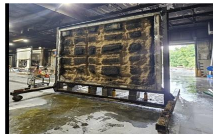
Hempcrete Product Passes Fire Resistance Testing [14]
